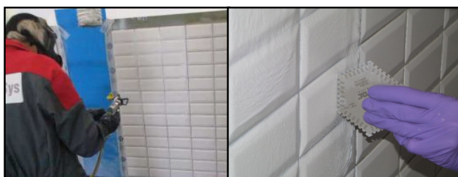
FIG. 9: Large-scale spraying test of the biocide gel
