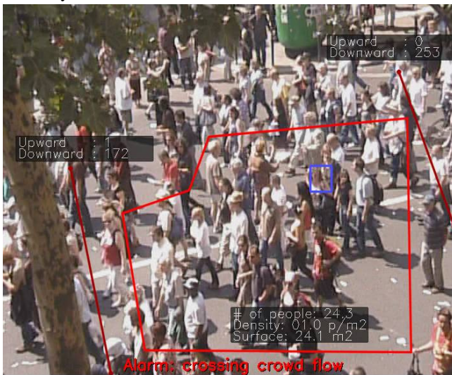
FIG. 6 : : (a) simultaneous density estimation, counting, and detection, (b) speed and direction
