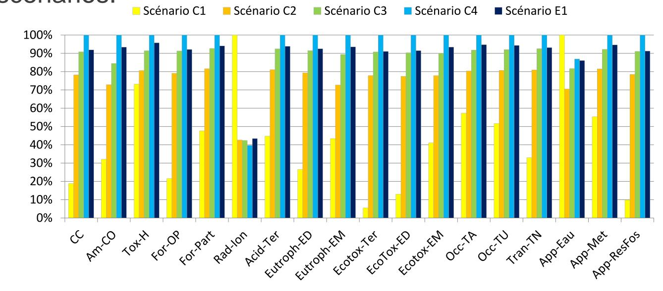
Result have shown that precipitation have the high impacts, respectively because of the ethanol fabrication and the energetic consumption. The scenario C1, which is the one without precipitation appeared to be the best in the majority of impact categories.
