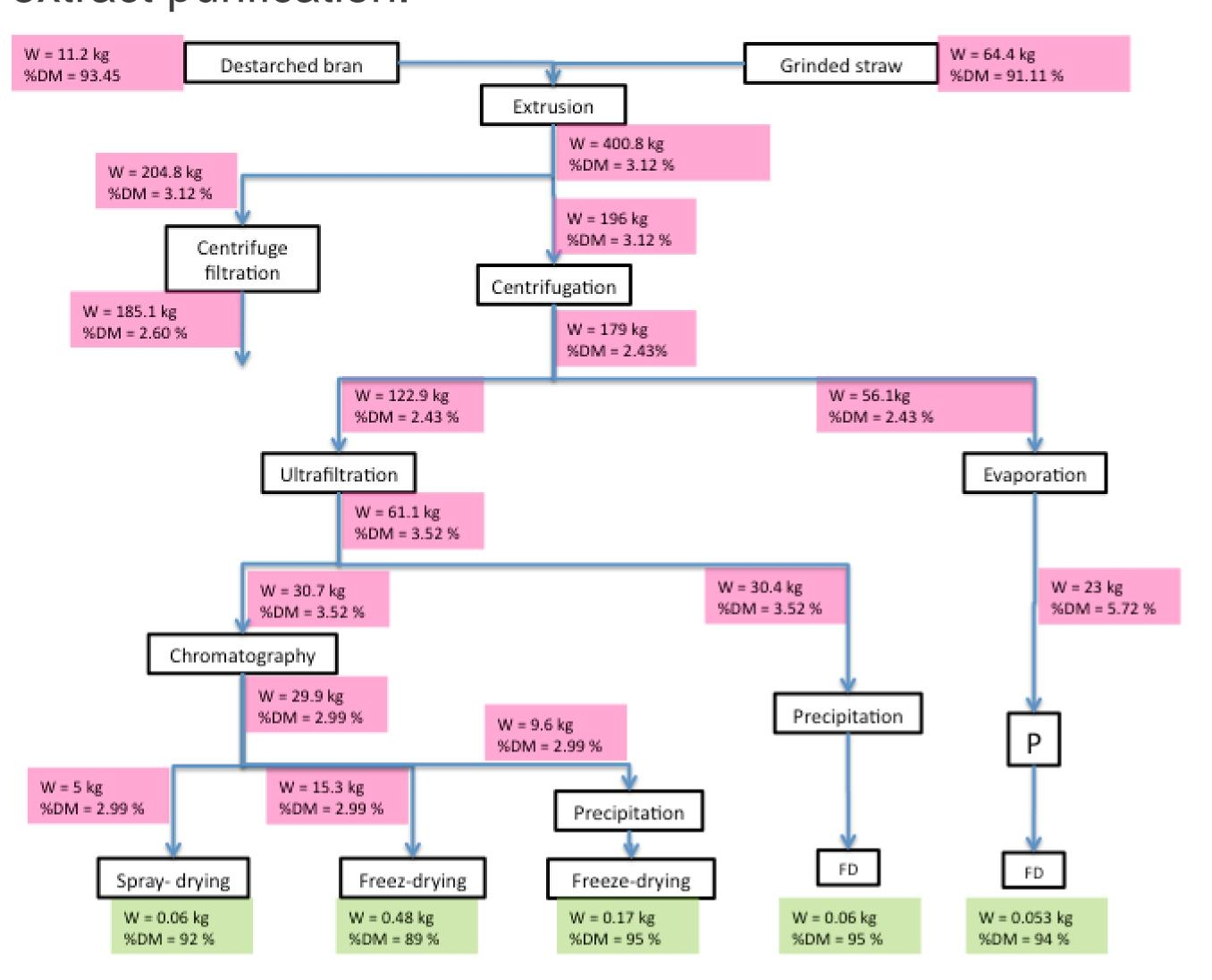
Centrifugation is more efficient than filtration for liquid/solid separation while ultrafiltration allows for both concentration and partial purification of the extract.
