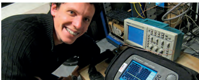
N Quintin observing the first stabilised optical signal arriving at the RENATER node hosted at the University of Strasbourg IT department. The very narrow spike on the screen is the first sign of the successful arrival in Strasbourg of REFIMEVE+. (2015)
