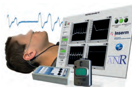
The PASITHEA system consists of a mobile recording device, a kinaesthetic stimulation system and a signal processing and real-time control application (1) .
